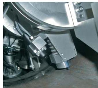
The suction units are based on the same principle as the grinding robots. The suction hose is connected with the motor radial positioning so that it is possible to specifically approach every point in the pipe and apply suction.
