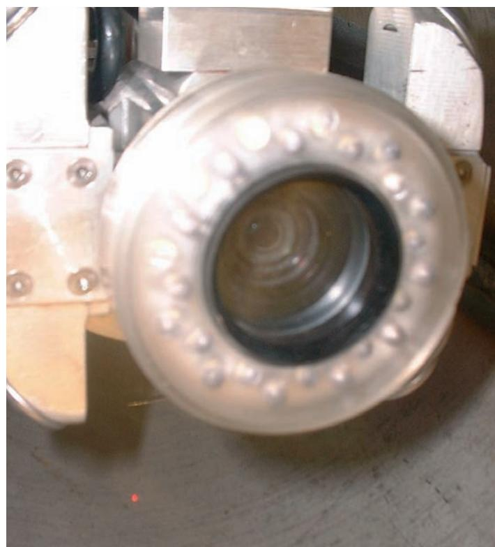
pan/tilt head. The point laser allows defects of > 2 mm to be measured. Its precision is better than 0.1 mm.
